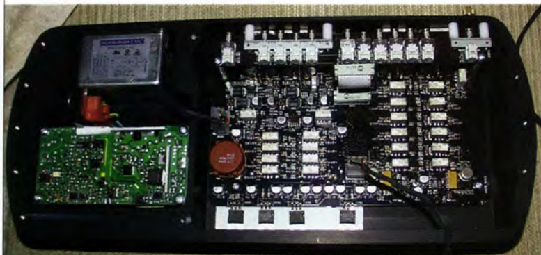
Chord Symphonic's relay rich innards. Note isolated power supply on left.
